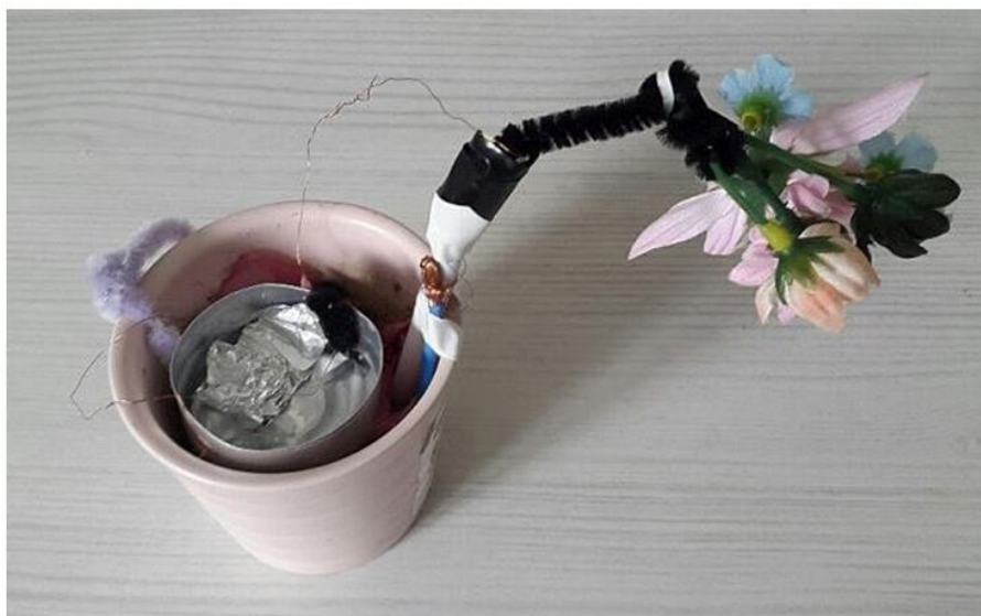
Figure 1: Battery poy with WFB-capacitor, c.f. [1], metal cup (NPN-diode) collecting Solar Heat and electrodes in bog moss (not visible)
