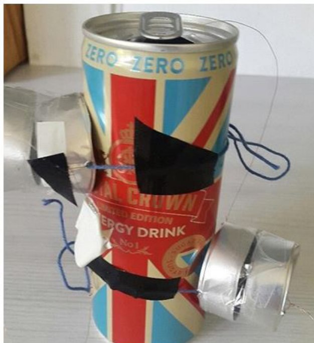
Figure 3: Two Heat Chambers on a can filled with hot water. The can acts as a bus distributing heat to the inner cup of the Chamber
